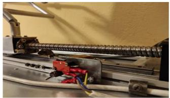
Figure 14. Mounting the limit switches.
