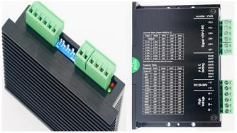
Figure 3. Motor Driver Nema 23 [6].
