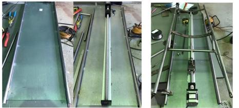
Figure 10. Mounting the motor and linear platform. Figure 11. Welding the support.
