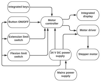
Figure 1. CPM device block diagram.
